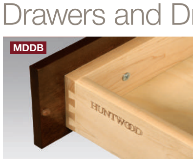
5/8" Solid Maple Dovetail Upgraded 5/8" thick solid Maple drawers with 1/4" thick captive bottom. Drawer fronts receive permanent bumper pads.
