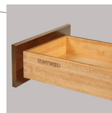
5/8" hardwood drawer box Natural finish and dovetail construction. Fully captive bottom is secured by side dados. Soft-close feature included.
